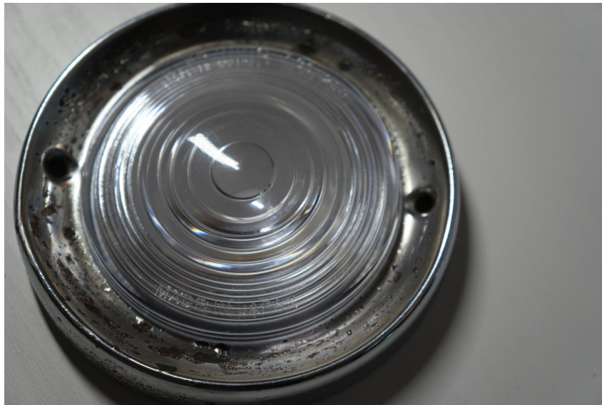
2. Lens pressed in and oriented so the text reads upright.
